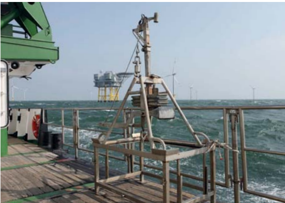
Images above: Sediment is lifted from the seabed with a box grabber.
