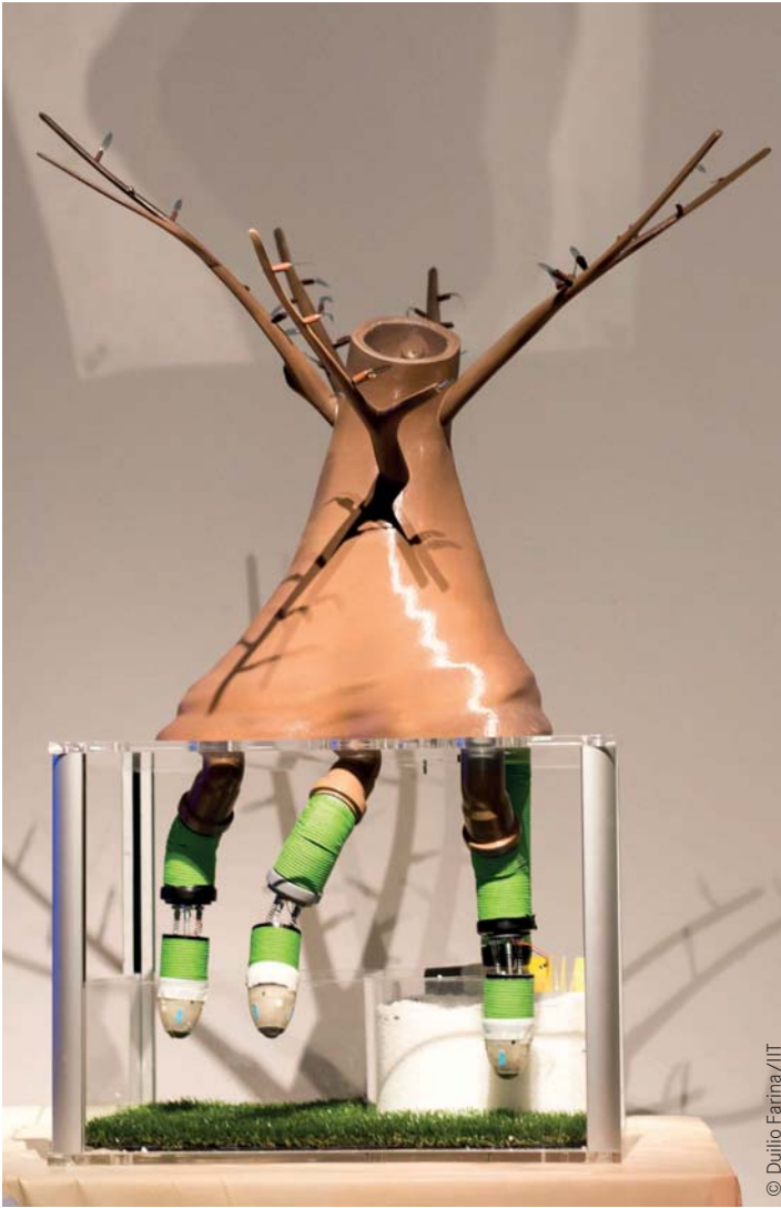
The scientists at IIT have developed a plantoid, a robot that behaves and grows like a plant. It serves the investigation of biological and technological questions.
