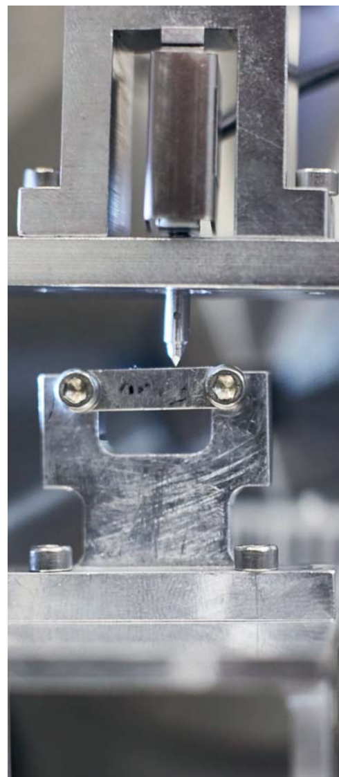
The positioners push the sample into the tip of the indenter with a defined force (right hand image).
